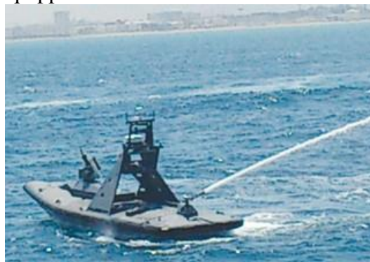
Picture 4: Israeli USV equipped with water cannon [5]
